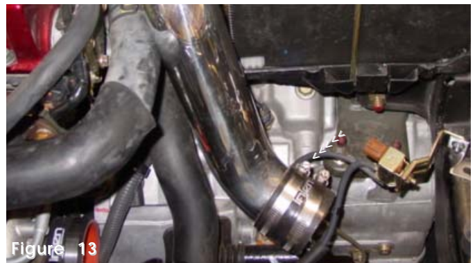
Figure 13 Press the 2 1/2" straight hose over the end of the intake and use two .312 power-bands, tighten the band on the intake.
