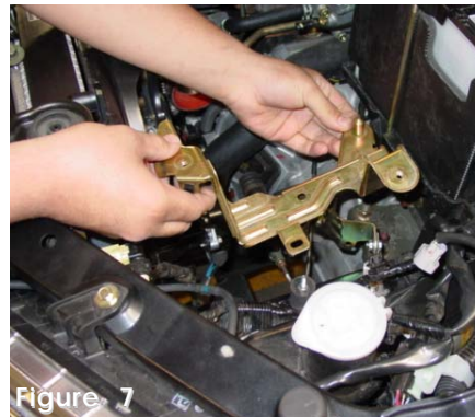
Figure 7 Remove the stock zinc plated brace that once held the air intake box and boost solenoid in place.
