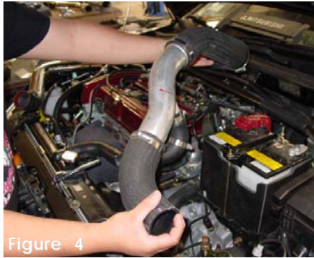
Figure 4 Remove the stock intercooler piping with the rubber with the stock hose connectors. The piping to the driver side front intercooler is removed with the exception to the connecting hose on the intercooler.
