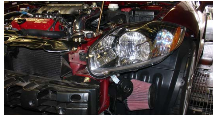
Once the entire cold air intake has been installed, adjust for best possible fit. Once the intake has been cleared from rubbing and rattling continue to tighten all nuts, bolts and clamps. Periodically, check for rubbing, leaks or rattling along the length of the intake in order to avoid damage to the intake.
