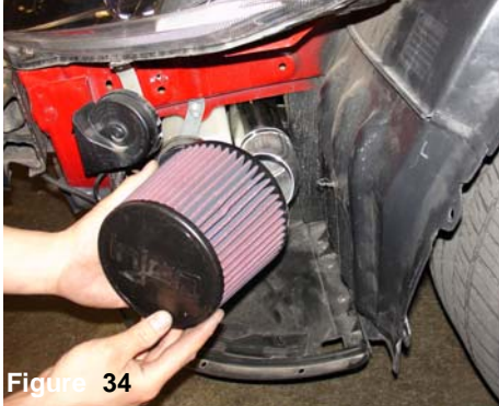
Figure 34 Press the filter over the end of the secondary intake. Once the intake end is butted up to the filter stops, continue to tighten the filter neck clamp.
