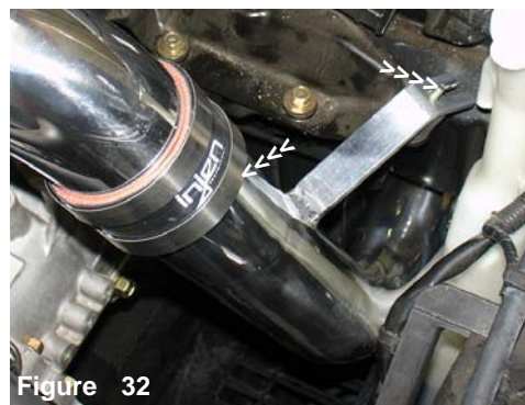
Figure 32 Press the upper end of the intake into the 3" straight hose while aligning the intake bracket to the vibra-mount.
