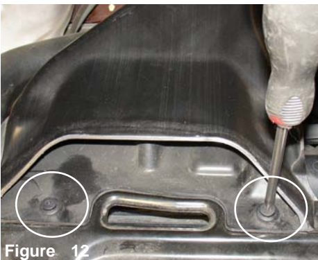
Figure 9 Once you have removed both screws, continue pulling out the mass air flow sensor from the sensor housing.
