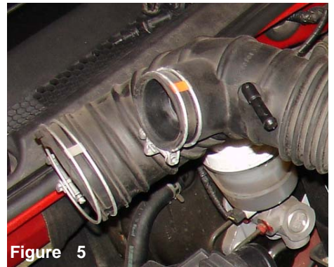
Figure 4 The throttle body and resonator clamps are loosened.
