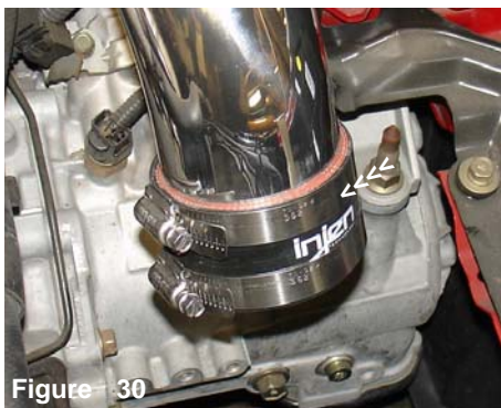
Figure 30 Press the 3" hose over the end of the primary intake. The 3" hose should not cover more than 1" of the edge of the intake. Use two power-bands and tighten the clamp on the intake side for now.
