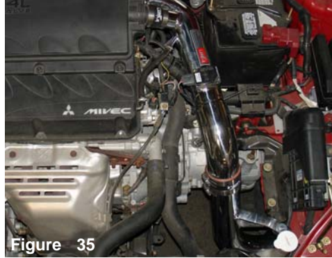
Figure 32 Press the upper end of the intake into the 3" straight hose while aligning the intake bracket to the vibra-mount.
