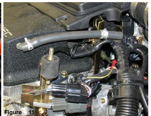
Figure 11 The vibra-mount is screwed into the bracket until it is flush to the zinc plated bracket.
