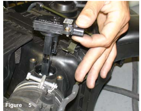
Figure 5 Carefully pull the mass air flow sensor from the air sensor housing as shown above.
