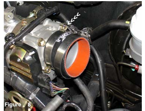
Figure 8 Press the 2 7/8" straight hose over the throttle body. Place two power bands (.362) over the 2 7/8" hose and tighten the clamp located over the throttle body.
