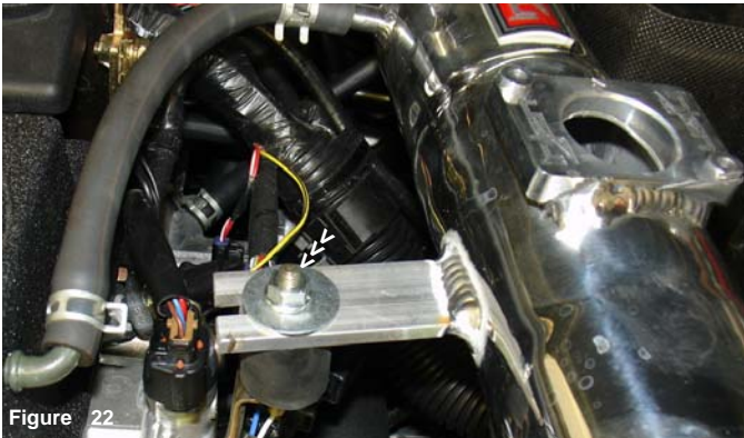
Figure 22 Use the m6 flange nut and fender washer to secure the intake bracket to the vibra-mount>
