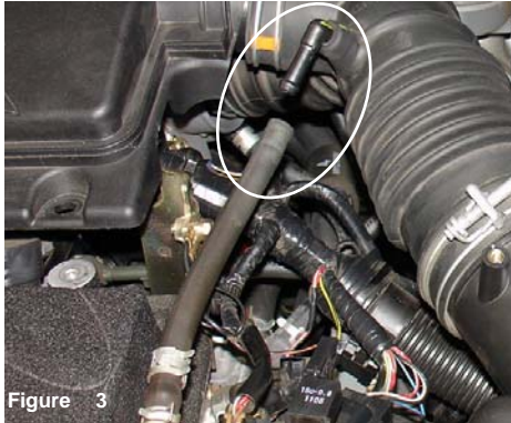
Figure 3 Disconnect the vacuum line from the rubber air intake duct.
