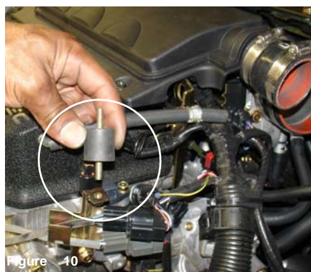
Figure 10 Align the vibra-mount to the gold zinc plated bracket located to the side of the valve cover.
