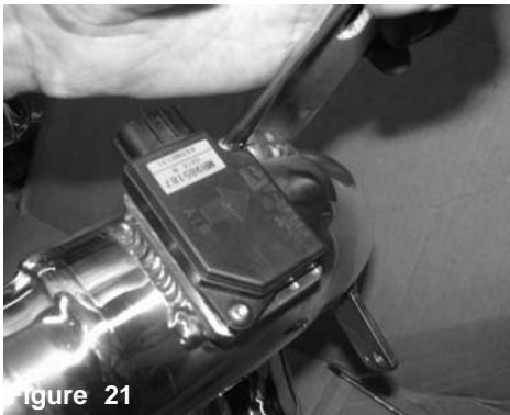
Figure 18 The two mass air flow sensor screws are loosened and removed from the sensor housing.
