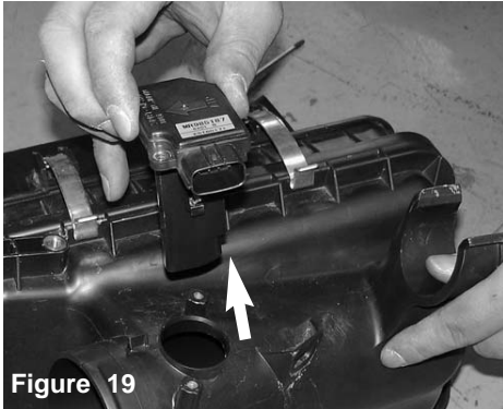
Figure 20 Install the MAF sensor into the new intake tube
