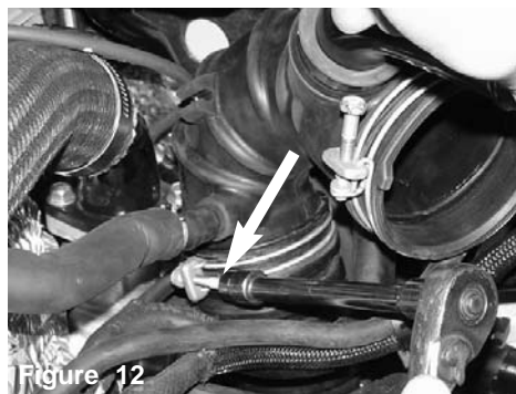
Figure 9 The blow off return line clamp is loosened prior to removing the air box. The hard line is removed from the intake tube.
