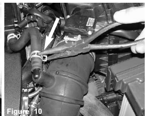
Figure 7 The air scoop is dislodged and pulled from the opening of the air box cleaner as shown above.
