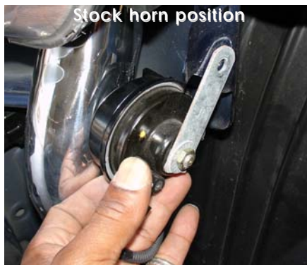
The stock horn is removed from its stock location and is turned around to keep intake from rattling.
