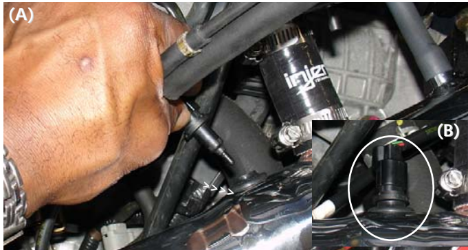
Press the air temperature sensor in to the 1525 sensor grommet (A). Insert the air temperature sensor into the grommet until it bottoms out (B).
