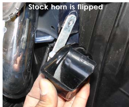
Turn the horn around so that it faces outward. Position the horn in place and screw the bolt back into the bumper frame.
