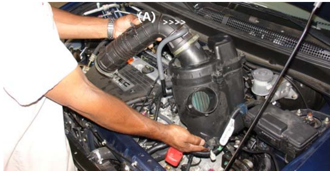
Loosen clamps and bolts in order to remove the air intake duct and air intake box from the engine compartment. Prior to pulling the air box out, remove the 8mm breather hose (A).
