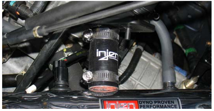
Here, the air temperature sensor, CCV hose, CCV box, and breather lines have been installed and completed.
