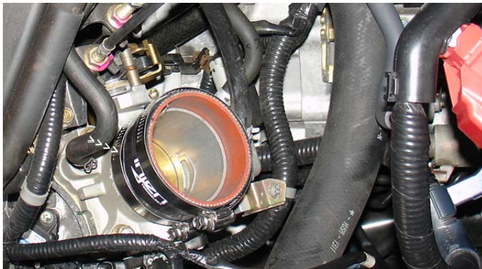
Press the 2 3/4" straight hose over the throttle body, place two Power-bands over the hose and tighten the hose on the throttle body side.
