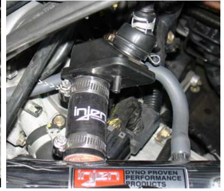
Once the CCV box has been correctly installed continue to tighten the mini-clamp.
