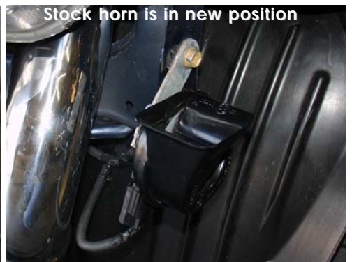
The screw is tightened into the bumper frame and the horn is now relocated.
