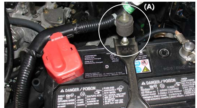
Screw the female vibra-mount over the battery post (A). Usually, 8 complete turns will be enough to level the intake bracket.
