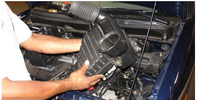
Note: For this installation, it will be required to remove the front bumper. Once the bumper has been removed continue to remove the stock air intake resonator from the bumper area.
