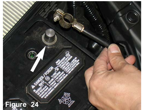
Figure 24 Disconnect the negative battery terminal
