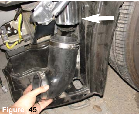
Figure 45 With the primary pipe exposed in the air box resonator area, Place the long side of the 90 degree hose (X-3144) over the end of the primary intake. Also place two .056 clamps (X-4005) onto the hose.
