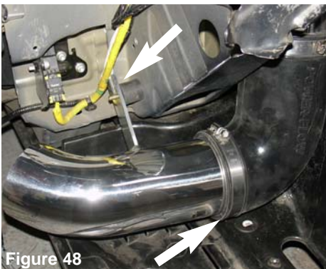
Figure 48 The secondary intake bracket is attached to the vibra-mount stud. The intake is firmly placed into the 3 1/2" 90 degree elbow.
