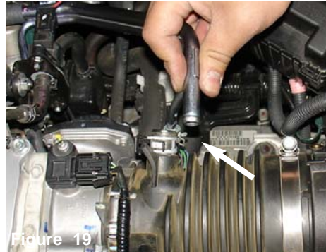
Figure 19 Pull the steel PCV breather tube out of the factory air box duct.
