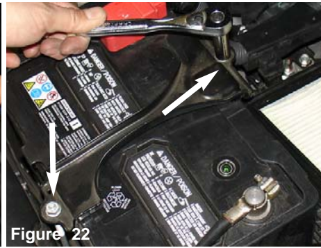
Figure 22 Using a deep 10mm 3/8 socket and ratchet, loosen the two 10mm nuts from the battery tie down.
