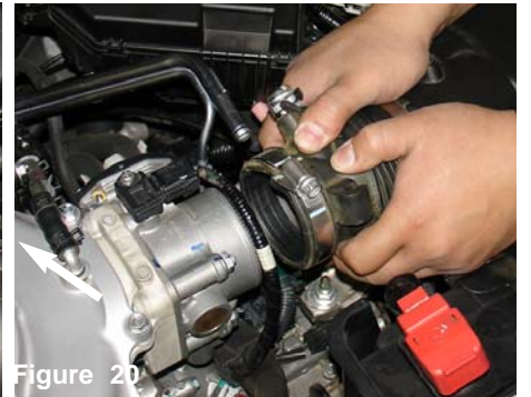
Figure 20 Disconnect the air box duct from the throttle body.
