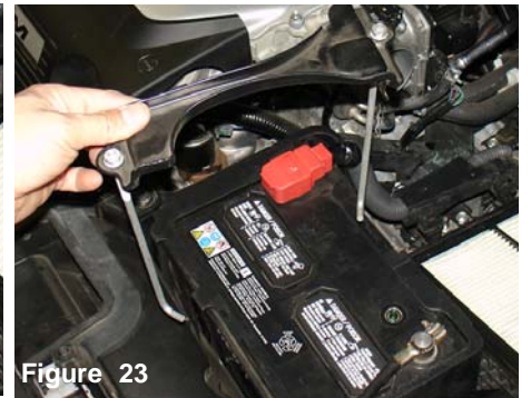
Figure 23 Now remove the battery tie down.
