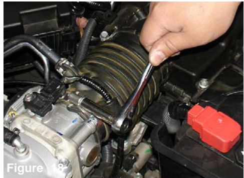
Figure 18 Use a 10mm 3/8 socket and ratchet to loosen clamp on the factory air box duct
