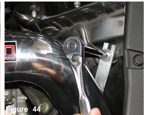
Figure 44 Use a 10mm 3/8 socket and ratchet to tighten the M6 nut to the vibra mount.
