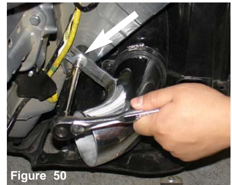
Figure 50 Use a 10mm 3/8 socket and ratchet to tighten the M6 nut.
