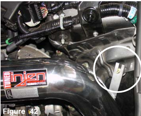
Figure 42 Line the primary intake bracket to the vibra mount stud located on the shock tower mount.
