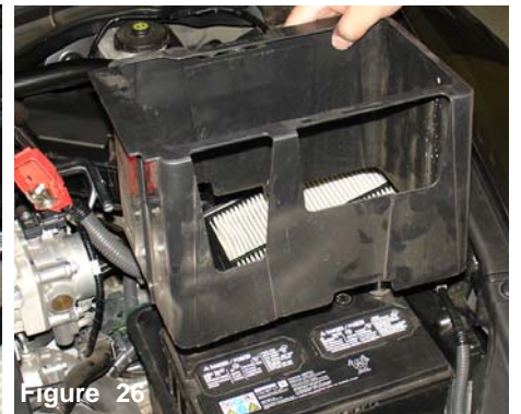
Figure 26 With the battery terminals disconnected, you can now remove the battery heat cover.
