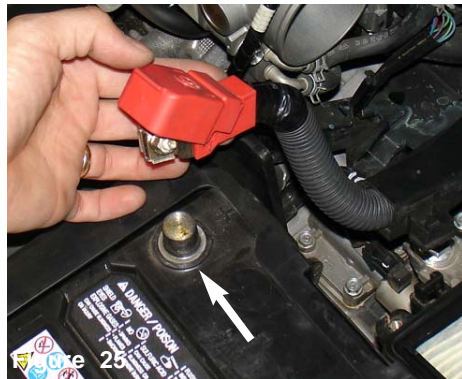
Figure 25 Now disconnect the positive battery terminal.
