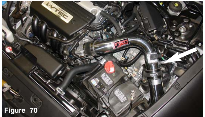
Figure 70 Congratulations! You have just completed the installation of this intake system. Periodically, check the alignment of the intake, normal wear and tear can cause nuts and bolts to come loose. Failure to check the alignment and adjust the intake can cause damage that will void the warranty.
