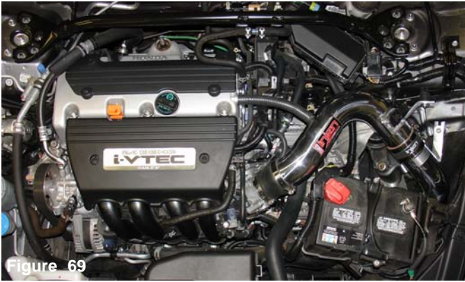
Figure 69 Align the entire intake for best possible fit. Once you have aligned and made sure that the length of the intake is free from any moving parts, continue to tighten all nuts, bolts and clamps.
