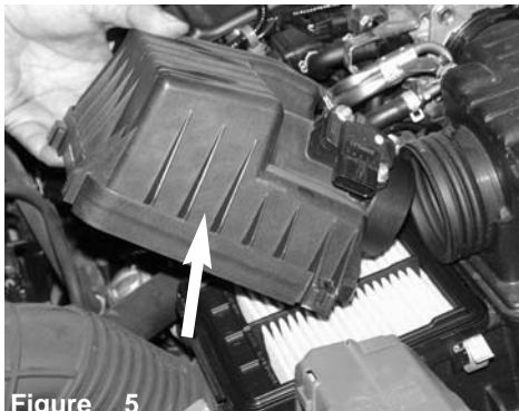
Figure 5 Un-clip the upper half of stock air box and lift and pull of vehicle. Remove stock air filter.
