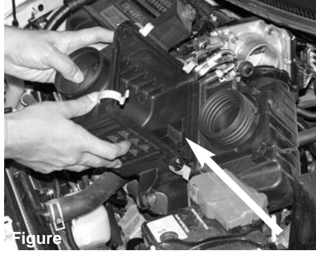
Figure 9 Carefully lift and remove the stock air box out of vehicle.
