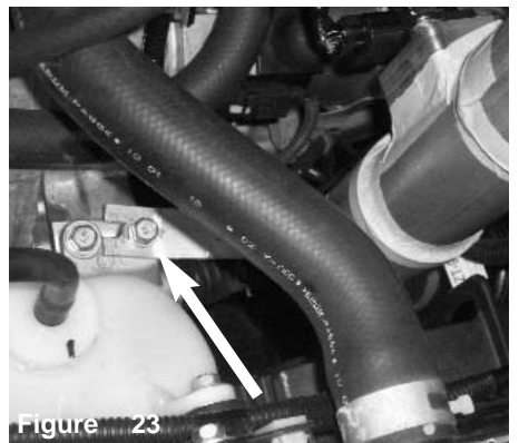
Figure 23 Install the elbow coupler with clamps to throttle body. Position the intake assembly into the vehicle.
