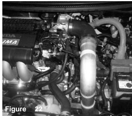
Figure 22 Tighten all the clamps on the intake tube using 8mm nut driver.
