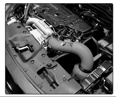
Congratulations! You have just completed the installation of this intake system. Periodically, check the alignment of the intake, normal wear and tear can cause nuts and bolts to come loose. <u>Note: Check clearance and adjust if needed! Failure to check</u> the alignment and adjust the intake can cause damage that will void the warranty. Injen Technology is not responsible for any damages caused by/from improper installation.
