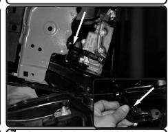
**7.** Loosen the 1 screw holding in the resonator bracket. Remove the bracket from the vehicle.
