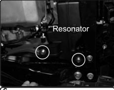
**6.** Now with vehicle on a lift or on jackstands secured, remove front bumper cover. From under the vehicle, pull back splash guard, loosen the 2 bolts holding in the resonator box.
