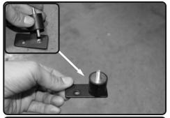
**11.** Now install the M6 vibramount to the thredded fitting on the provided bracket. Secure and tighten.
