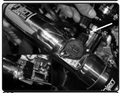
**16.** Install the MAF sensor into the machined pad. Secure using 2 two screws from step 4.
