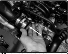
**13.** Install the 2-3/8" straight hose with clamps to the turbo housing. Tighten the clamp on the housing only.
