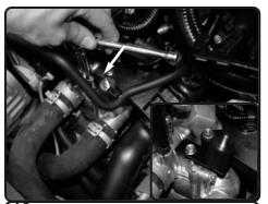
**12.** Now install the new provided bracket to the engine, secure using the original screw. Tighten using 10mm socket or wrench.
