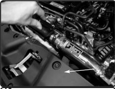
**18.** Tighten the clamp on straight hose.
