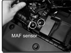
**3.** Using phillips screwdriver, loosen the 2 screws holding in the MAF sensor.
