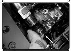
**20.** Install the 2-3/4" straight hose with clamps to the upper intake assembly
