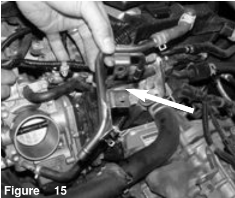
Figure 15 Remove the complete coolant and crank case assembly from engine.
