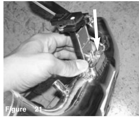
Figure 22 Using the factory screws, secure the MAF sensor.
