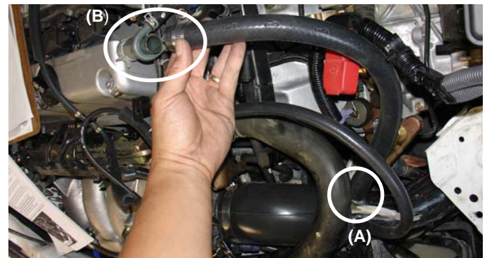
Take the 18" 17mm vacuum hose and press one end over the 3/4" intake port (A). Press the other end over the crankcase port (B), use the small clamps in this kit to secure the hose at the crankcase and the intake port.
