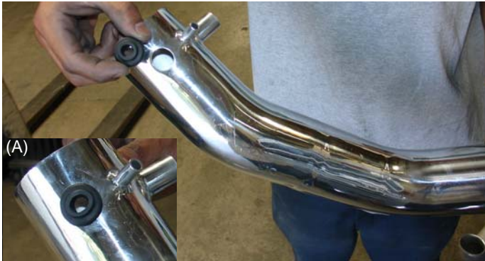
Take the 1525 sensor grommet and press it into the pre-drilled 3/4" hole as shown in (A). Insert the grommet into the hole until grommet is well seated throughout the hole circumference.
