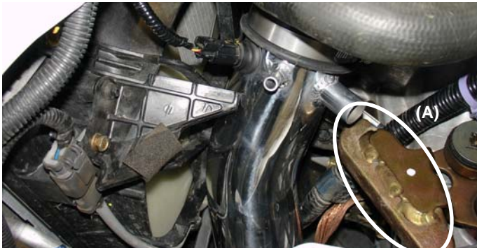
In 5th gear, the shift lever link should be facing the intake. Adjust the intake so that it is away and free from hitting the lever (A). Press the upper portion of the intake into the elbow with the clamp.
