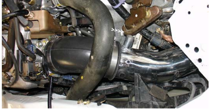
Once the intake has been aligned for best possible fit have a second person shift through all the gears to make sure that the intake does not obstruct the shifting in anyway. If the lever does not hit the intake continue with the installation of the intake.
