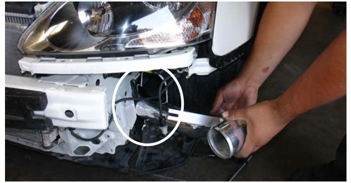
Install the upper portion of the intake through the bumper opening. Bring it up into the engine compartment and into the throttle body elbow.
