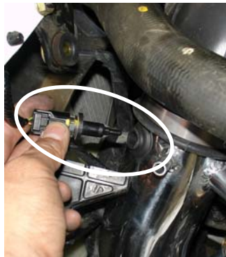
Locate the air temperature sensor and press it into the 1525 sensor grommet.
