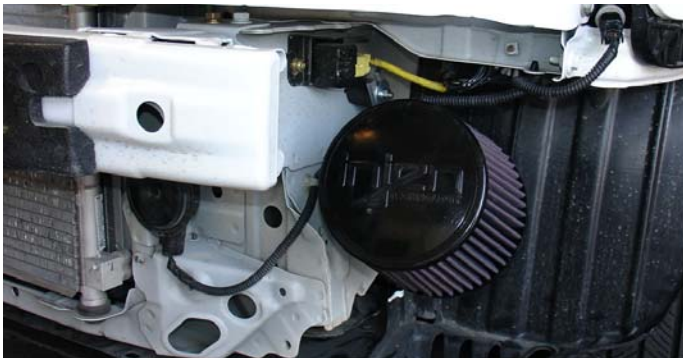
Take the filter and press the filter neck over the end of the intake. Use the clamp on the filter neck to secure the filter to the intake.
