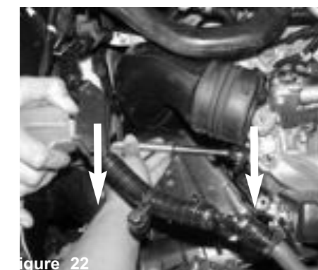
Figure 22 Remove the two lower 12mm bolts from the battery support bracket attached to the chassis
