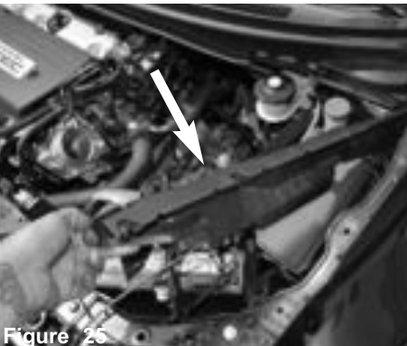
Figure 25 Remove the plastic side cover inside the engine compartment. Release the push clips to remove.
