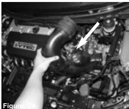
Figure 24 Pull firmly on the lower resonator duct to detach it from the resonator box located in the front bumper. This air duct will no longer be used.
