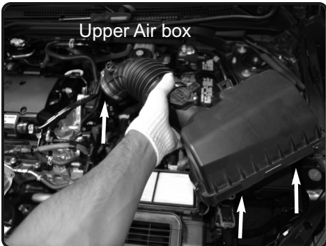
4. Unclip the upper half of the airbox, and remove from the vehicle.
