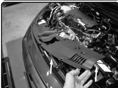
5. Remove the plastic push clips from the front plastic cover above the radiator. Remove plastic cover.
