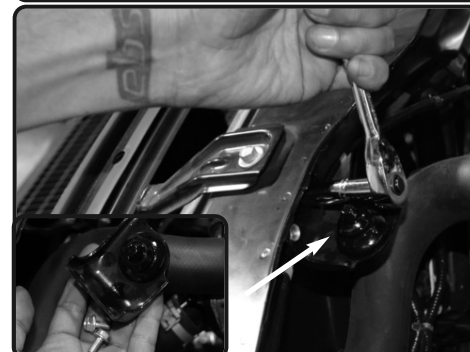
7. Loosen the OEM air box bracket out of vehicle using 10mm socket or wrench. Save 1 screw for later install.
