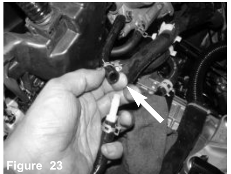
Figure 20 Loosen the clips on the hard line and slide back. This will be removed and secured with a 1/4" vinyl coupler. Note: Place a shop rag under neath and make sure vehicle is cold and not warm, there will be some coolant leaking.
