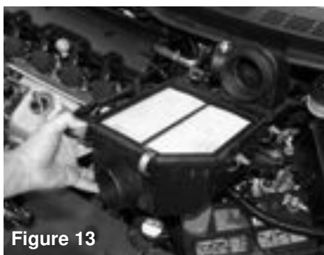
Figure 10 Firmly pull the rubber air duct off the front of the lower air box assembly.
