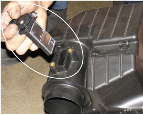
Unscrew the two screws that hold the mass air flow sensor to the housing unit.
