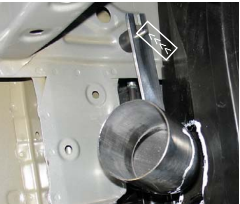
As the secondary intake is butted up to the primary intake, the intake bracket is also lined up to the vibra-mount stud.
