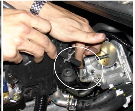
Take the Injen 15"-6mm braided vacuum hose and press it over port. Use the tension clamp to reconnect and secure the hose in place.
