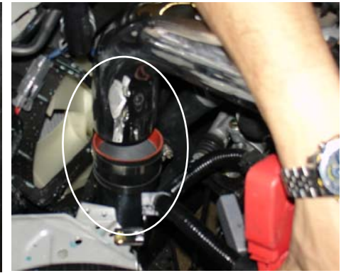
As the secondary intake is raised into the engine compartment, press the 3 inch hose over the end of the primary intake.
