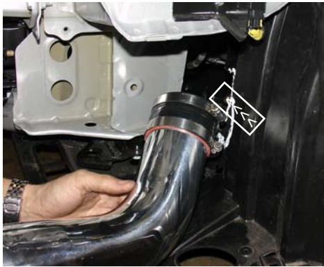
Insert the end with the 3 inch straight hose into the pre-cut hole and gently push it into the engine compartment until it connects with the primary intake.
