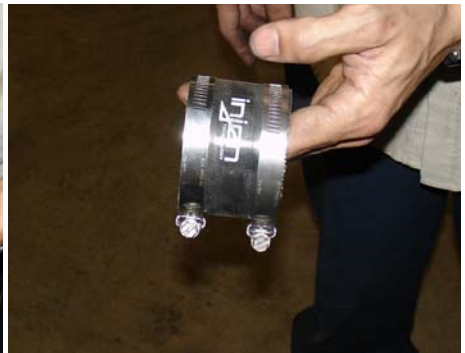
Place two clamps on the 2 1/2" straight hose as shown above.
