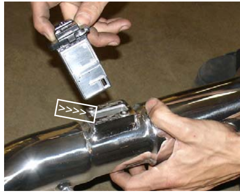
Checking the direction of the air flow sensor, insert sensor into the machined air flow adapter as shown above. Use stock screws to secure the sensor to the machined adapter.
