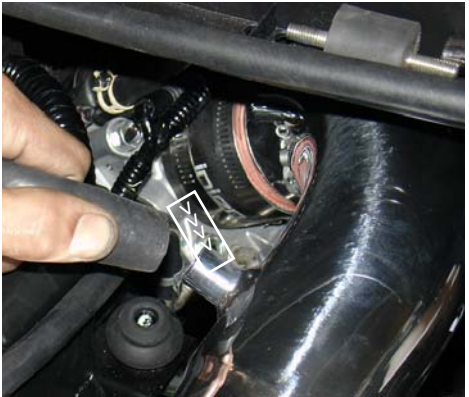
Press the other end of the 6" vacuum line over the intake port as shown above.
