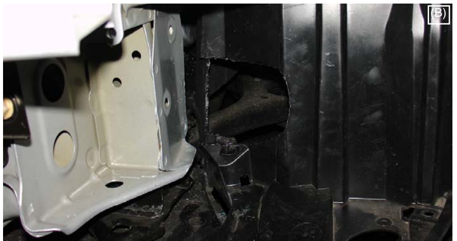
A small 4" cut away section is cut out of the plastic splash guard as shown above. The cut away is in a form of a "C", three sides are cut out (A). Clearance has been made and the secondary intake is now ready to be installed (B).
