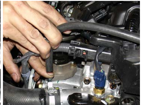
Now press the other end of the 15"-6mm hose coming from the throttle body, over the port located on the upper coolant outlet. The finger over the port is used to stop coolant from splashing out.
