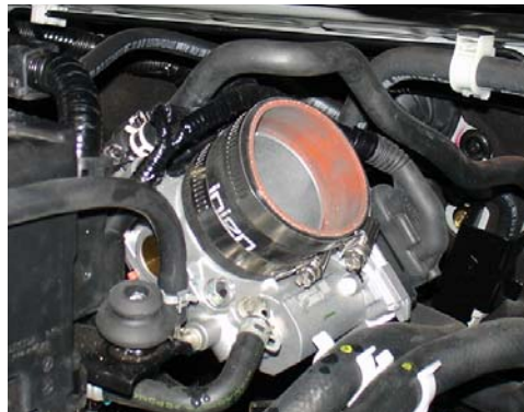
Press the 2 1/2" straight hose over the throttle body and tighten the clamp on the throttle body end.
