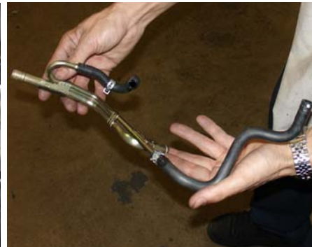
The PCV hard pipe is now removed from the stock coolant and breather lines.
