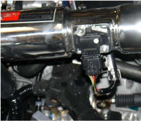
Close up of the air mass sensor connected to the machined adapter and the harness has been secured to the sensor.
