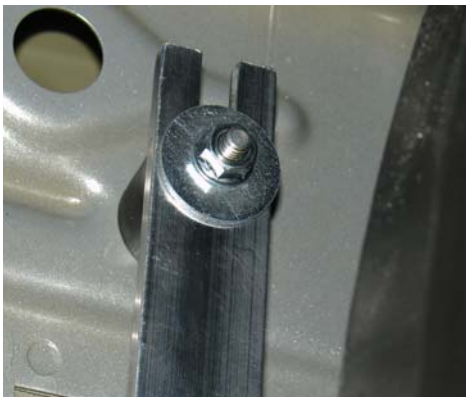
Once the intake bracket has been lined up to the vibra-mount stud, use the fender washer and flange nut to secure the intake to the vibra-mount.
