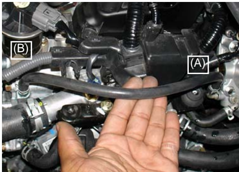
The 15"-6mm vacuum hose is now connected from the throttle body (A) to the upper coolant outlet port (B).
