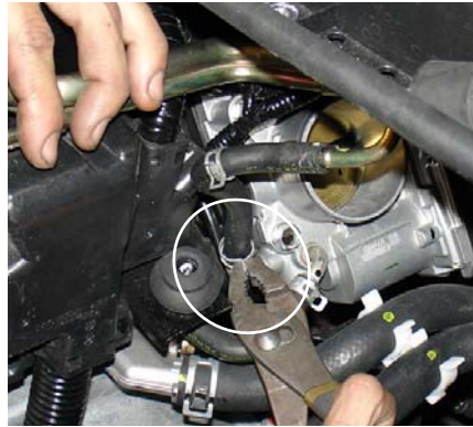
With pliers, remove the tension clamp connecting the coolant line running to the throttle body. Now remove the hose from the port.
