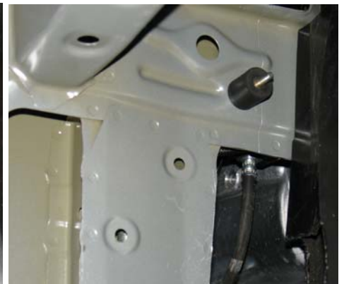
The vibra-mount is firmly sitting flush on the frame as shown above.
