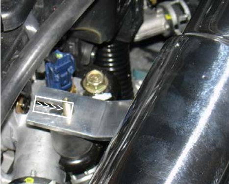
As the top end of the intake is inserted into the throttle body hose carefully align the intake bracket to the vibra-mount stud as shown above.
