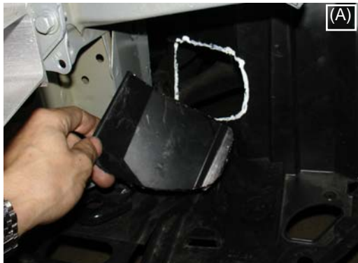
A small 4" cut away section is cut out of the plastic splash guard as shown above. The cut away is in a form of a "C", three sides are cut out (A). Clearance has been made and the secondary intake is now ready to be installed (B).
