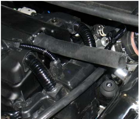
Press the 6"-17mm breather hose over the crank case port as shown above.
