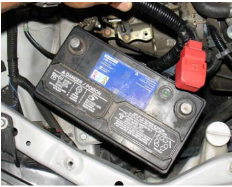
For this installation remove the negative and positive battery terminals, then proceed to remove the battery. Always place the battery on a table or cardboard paper in order to prevent grounding of the battery.
