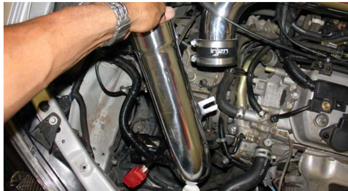
Once the filter has been installed on the secondary intake lower the filter end into the compartment below the battery tray.
