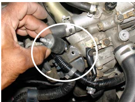
Screw the second vibra-mount into the brace next to the thermostat housing
