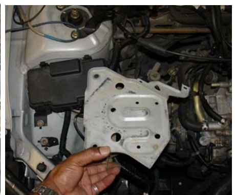
Once the battery has been removed continue to remove the plastic tray and metal battery tray.
