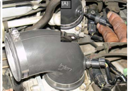
Take air temperature sensor and press it into the grommet located in the 90 degree elbow(A). The air temperature sensor is now installed.
