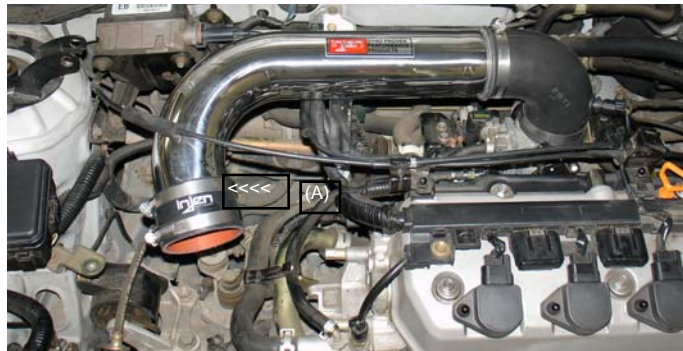
To continue the installation of the cold air intake take the 3" straight hose and press it over the end of the primary intake. Use two clamps on the hose but only tighten the clamp on the intake side (A).
