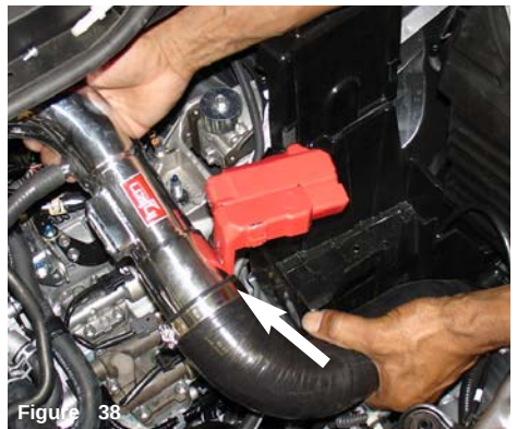
Figure 38 The silicone intake is pressed over the end of the intake.
