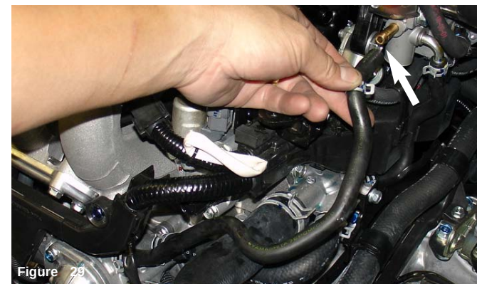
Figure 27 All lines have been removed or disconnected and the PCV hard line is now ready to be removed.
