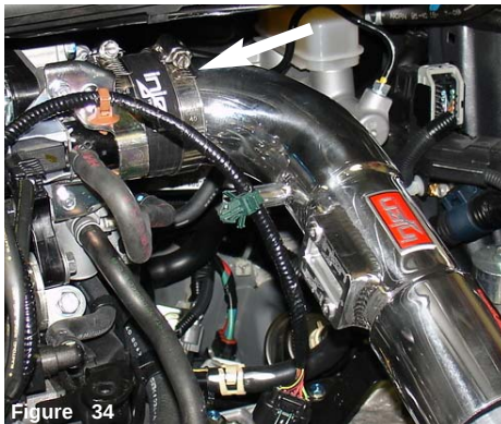
Figure 34 Press the primary intake into the throttle body hose as shown above, semi-tighten the power-band.
