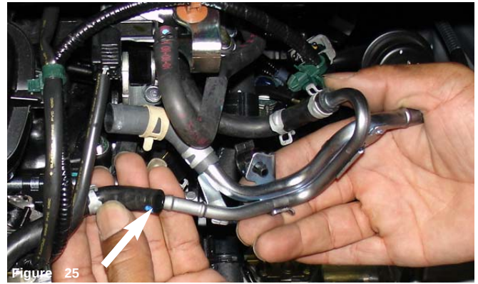
Figure 25 The lower coolant line is pulled from the PCV hard line.
