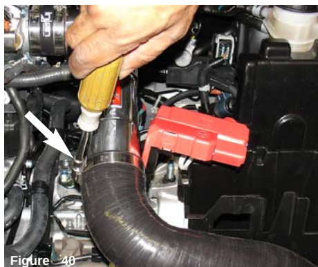
Figure 40 Approximately one inch of the silicone intake is pressed over the primary intake end. Once you have aligned the Primary intake to the silicone intake continue to tighten the Power clamp.
