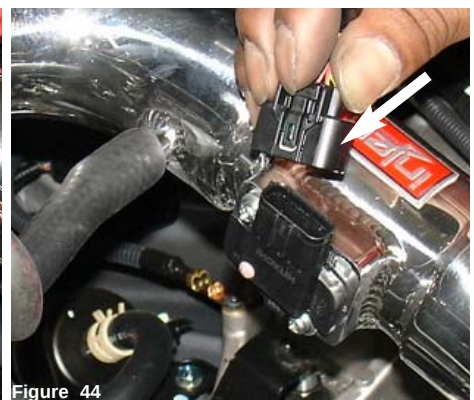
Figure 44 The electrical harness is pressed over the MAFS until it you hear them snap together.
