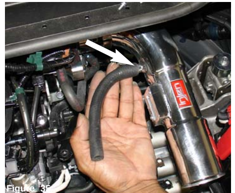
Figure 35 Press the 7" -10mm hose over the intake port.
