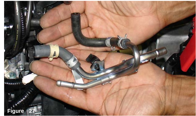
Figure 25 The lower coolant line is pulled from the PCV hard line.
