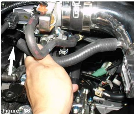
Figure 36 The other end of the 10mm hose is pressed over the crankcase vacuum port.
