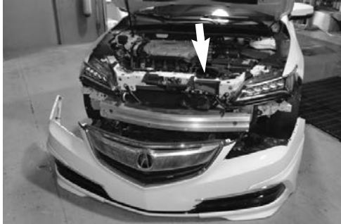
Figure 4 Front bumper cover needs to be removed from the vehicle for the factory resonator to be removed. Remove the plastic push-clips from top and bottom and remove side screws from the splash guard. Carefully pull back bumper cover. Disconnect Fog lights if equipped.
