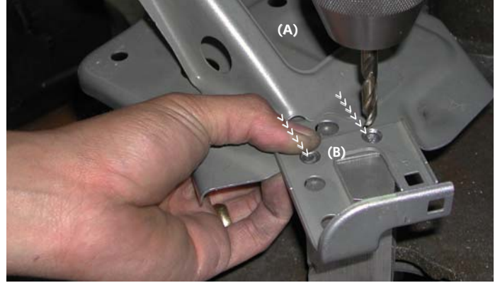
The battery tray is removed from the RSX (A). Turn the battery tray upside down and drill the two tacked or spot welded areas until the bracket becomes loose (B).
