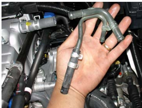
PCV hard pipe has been disconnected and removed from the breather hose and coolant lines.
