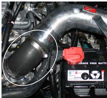
The primary intake is pressed into the elbow and the clamp is semi-tightened.
