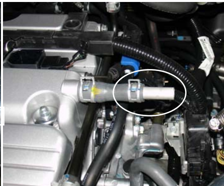
Insert the 1 1/2" long coupler into the crank case hose. Insert coupler half ways into the vacuum hose.
