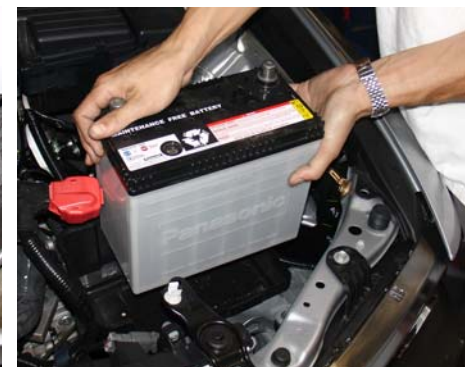
For best positioning of the cold air intake, removal of the battery will be required.
