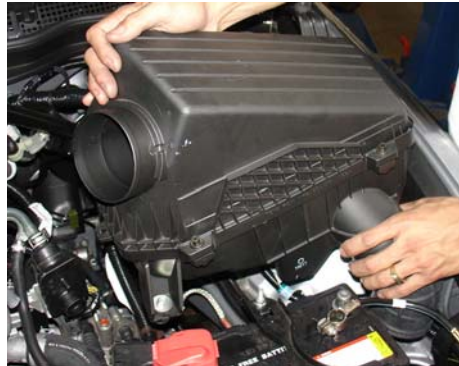
Loosen bolts and take out entire air intake box.
