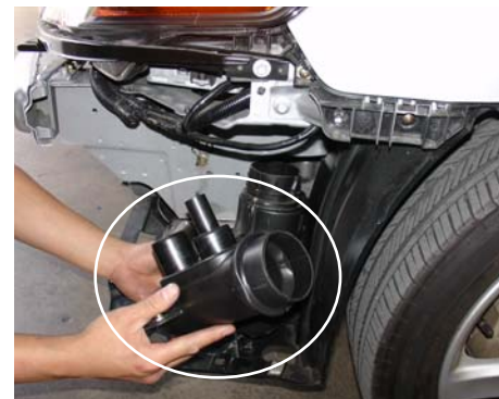
With the air resonator box out, remove the resonator connecting duct that connects the air resonator tube and air resonator box.
