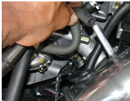
The stock injector solenoid breather line is inserted over the long 3/8" intake port as shown above.
