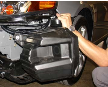
Note: In order to proceed to the next step, removal of the front bumper will be required. Loosen bolts and remove the air resonator box.
