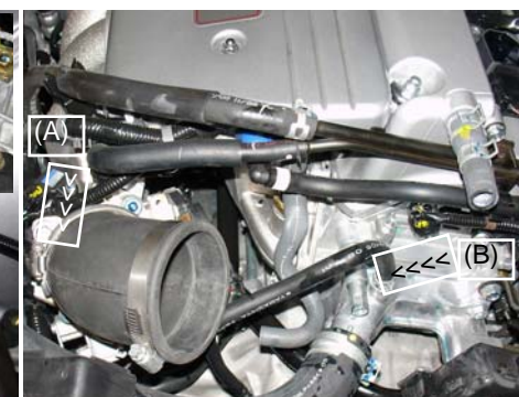
The 45 degree reducer elbow will slip over the 2 7/8" throttle body (A). Use two medium clamps and tighten the clamp on the throttle body side. The stock coolant line is installed over the coolant out port (B).
