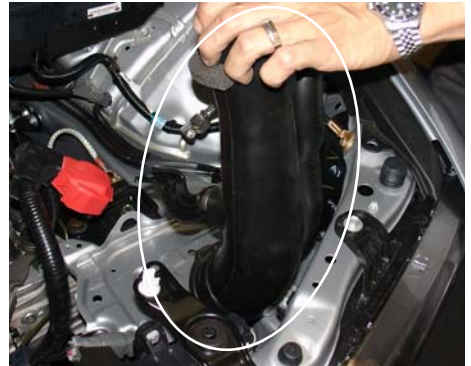
With the air intake box out of the way continue to remove the air resonator tube.
