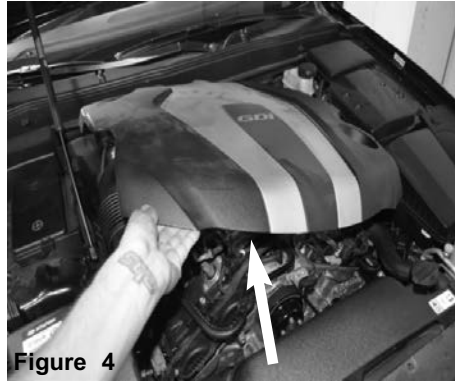
Figure 4 Lift up and remove the engine cover.
