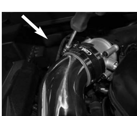
Figure 25 Tighten the clamp on the throttle body using 8mm nut driver.
