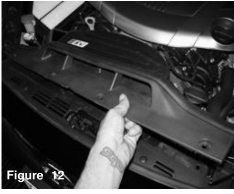
Figure 12 Remove the scoop, this will be used again in the new injen intake system.
