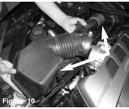
Figure 10 Un-clip the upper part of the air box and remove from the vehicle, including the resonator tube.
