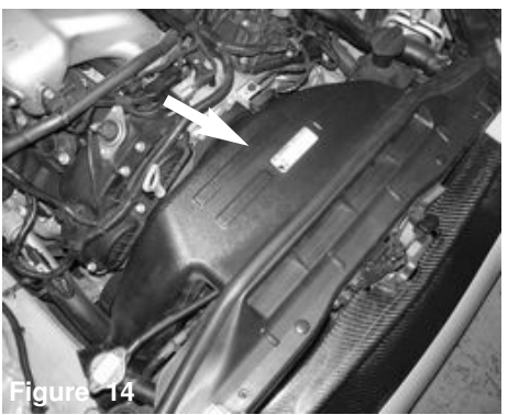
Figure 13 View of the stock air intake box and air intake duct.
