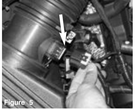
Figure 5 depress the tab on the electrical harness and gently pull on the harness clip.
