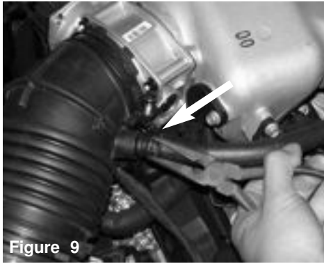
Figure 6 Loosen the clamp on the air intake duct as shown above.
