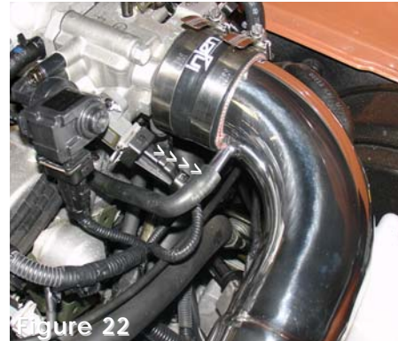
Figure 22 The vacuum hose is now installed.
