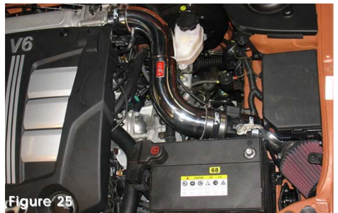
Figure 25 Align the entire intake for the best possible fit. Once you have position the intake to prevent any rubbing or rattling, continue to tighten all nuts, bolts and clamps.
