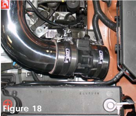
Figure 18 Lower the mass air flow sensor into the engine compartment and press it over the end of the intake as shown above.
