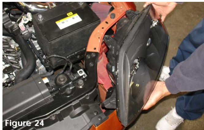
Figure 24 The head lamp is inserted into the head lamp cavity and restored to its original position.
