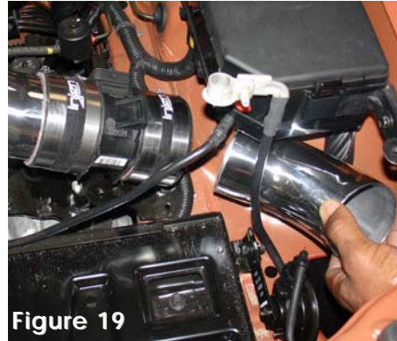
Figure 19 The secondary intake is then lined up the mass air flow sensor and inserted into the hose.
