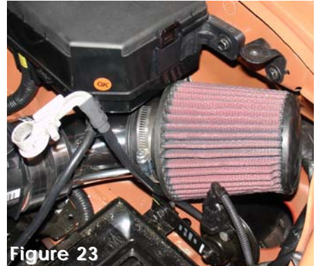
Figure 23 The filter is now pressed over the intake end and the filter neck clamp is tightened
