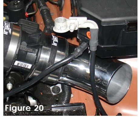
Figure 20 The secondary intake is now installed facing to the front of the car.
