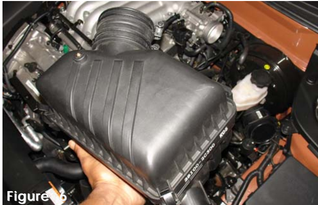
Figure 6 Once you have removed the three bolts from the lower air box, continue to remove the entire air box cleaner.
