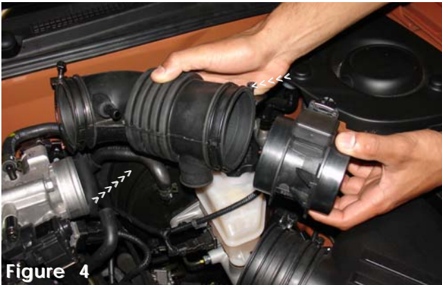
Figure 4 Once you have removed the entire air intake duct, continue to loosen clamp on the plastic air duct from the inlet side. Continue to pull the mass air flow sensor from the air intake duct.
