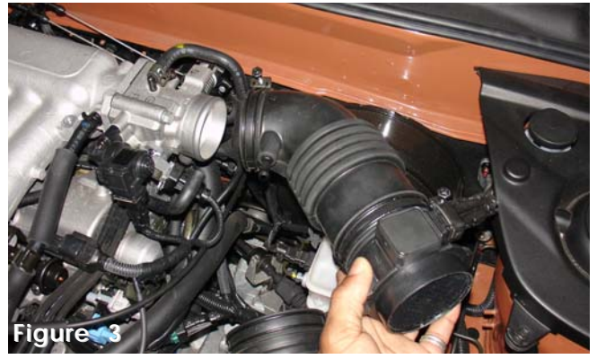
Figure 3 Once the clamp has been loosened from the throttle body and the air box cleaner, continue to remove the mass air flow sensor and air intake duct from the throttle body.
