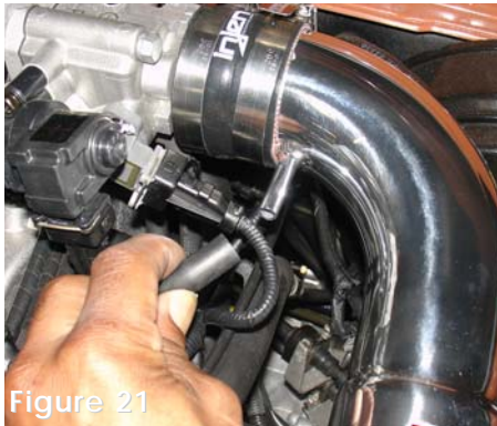
Figure 21 The stock air vacuum hose is lined up and pressed over the 3/16" intake port.
