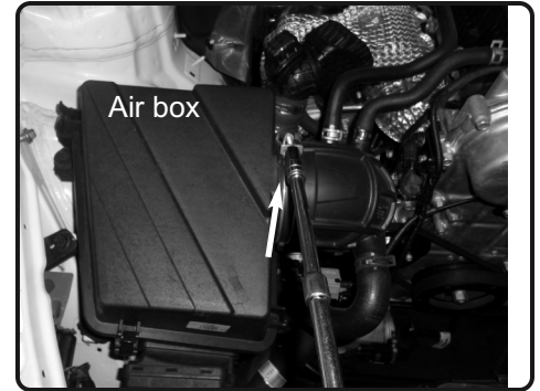
3. Loosen clamp on air box using 10mm socket or nut driver.
