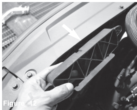
Figure 12 Loosen the 2 bolts holding in the front scoop vent and remove. Save 1 screw for later install.
