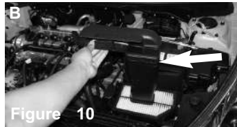
Figure 10 Figure A: Use a phillips screw driver and remove the two plastic screw clips from the front air intake duct Figure B: Lift up and remove the front air intake duct
