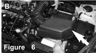
Figure 6 Figure A: Unclip the two tabs from the lower air box assembly to the upper air box assembly. Figure B: Detach the upper air box assembly from the lower assembly
