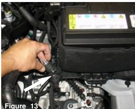
Figure 13 Screw the vibra mount onto the pre-threaded hole next to the battery
