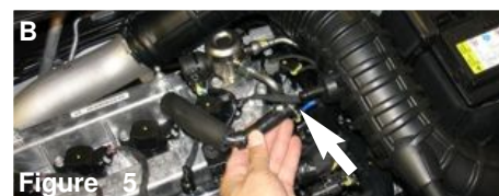
Figure 5 Figure A: Disconnect the recirculating diverter valve hose from the intake duct. Figure B: Disconnect the crank case breather line from the air duct.
