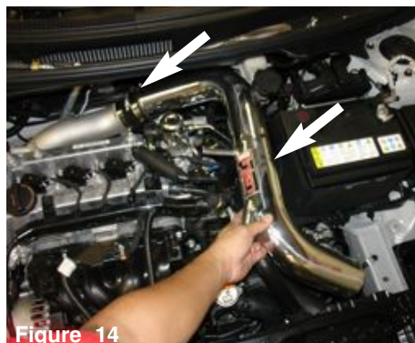
Figure 14 Position the intake pipe into the engine bay and place the end of the pipe into the step hose on the turbo compressor outlet.
