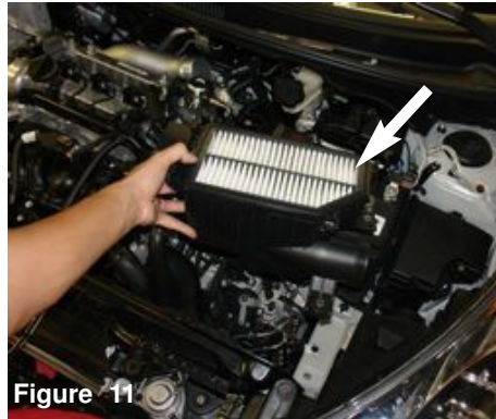
Figure 11 Now the lower air box assembly can be removed from the engine bay.
