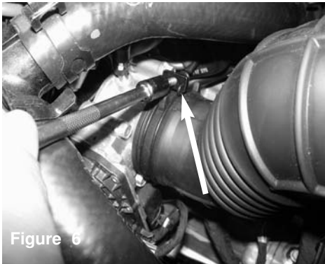
Figure 6 Use a 10mm socket/ratchet to loosen the clamp in the throttle body.
