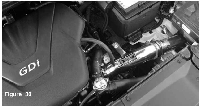
Figure 30 Congratulations! You have just completed the installation of this intake system. Periodically, check the alignment of the intake, normal wear and tear can cause nuts and bolts to come loose. Failure to check the alignment and adjust the intake can cause damage that will void the warranty.
