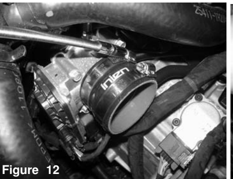
Figure 12 Install the step hose with clamps provided to the throttle body. Tighten the clamp on the throttle body using 8mm nut driver.
