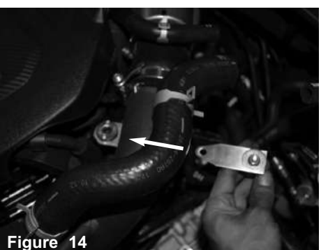
Figure 14 Lift the factory upper intercooler pipe up and slide the stainless bracket underneath the upper intercooler pipe bracket. Re-install the bolt from step 12.
