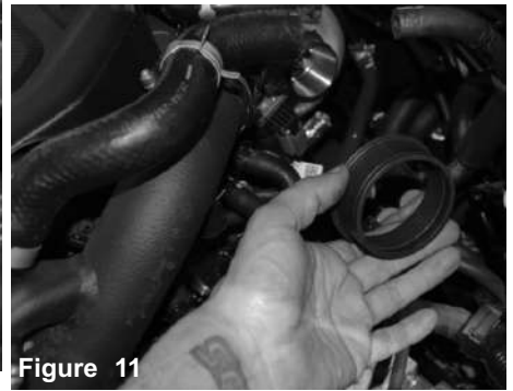
Figure 11 Remove the rubber coupler from the turbo.
