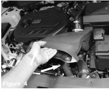
Figure 4 Use a 10mm socket/ratchet and remove the two M6 bolts attached to the factory air box inlet duct. Remove the air box inlet duct from the engine bay. This air duct will be re-used in this installation to draw in cool air to the Injen intake system.
