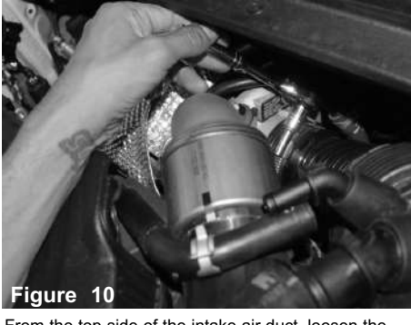
Figure 10 From the top side of the intake air duct, loosen the clamp with a 10mm socket/ratchet attached to the turbo inlet. Detach the intake air duct from the turbocharger and you may now remove the intake air duct from the engine bay.
