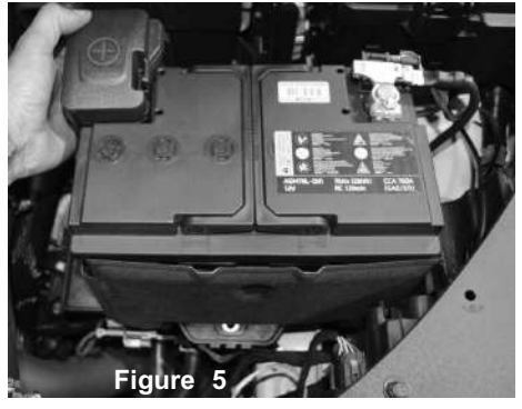
Figure 5 Loosen the battery bracket and pull battery forward. This will allow removal the the OEM air box.
