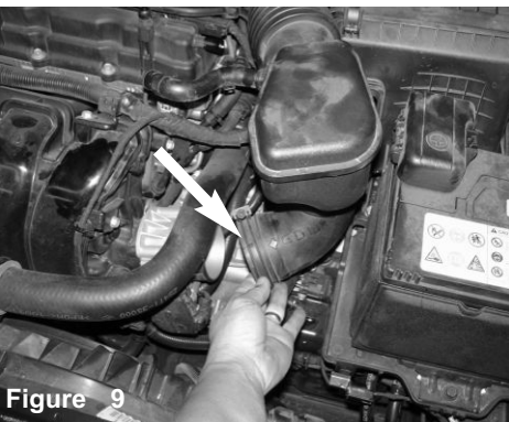
Figure 6 Use a plier to release the pressure clamp on the crank case vent tube on the OEM air duct. Disconnect the crank case vent tube from the vavle cover.
