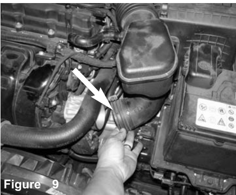
Figure 6 Use a plier to release the pressure clamp on the crank case vent tube on the OEM air duct. Disconnect the crank case vent tube from the valve cover.
