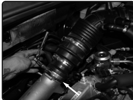
5. Loosen the clamp on the turbo housing using 10mm socket or wrench.
