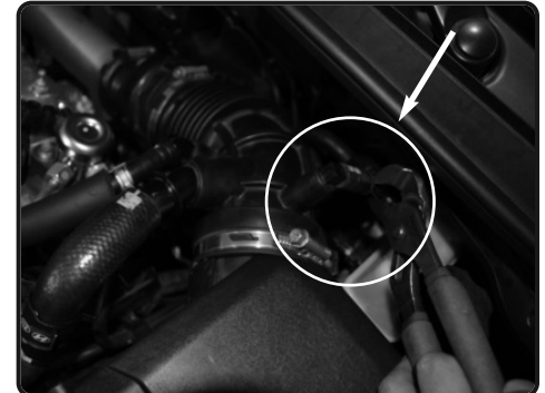
7. With pliers, pull back the vacuum line away from OEM intake tube.
