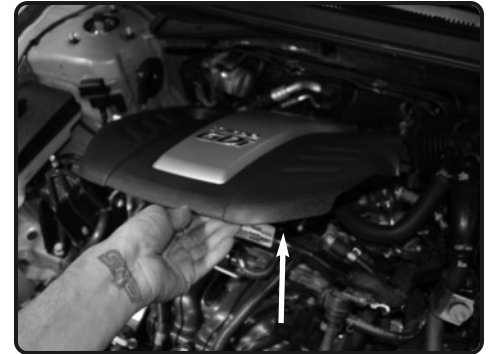
3. Lift up and remove the engine cover from the vehicle.
