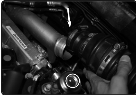
8. Lift up and pull back the OEM intake tube from the turbo housing.
