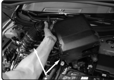
9. Now lift up and remove the factory air box from the vehicle.
