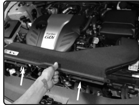
7. Now lift up and remove the factory scoop.
