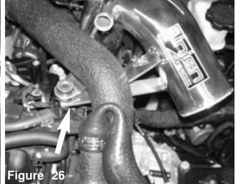
Figure 23 Remove the factory M8 bolt. This bolt will not be re-used in this intake installation. A longer supplied M8x40 bolt will be used.
