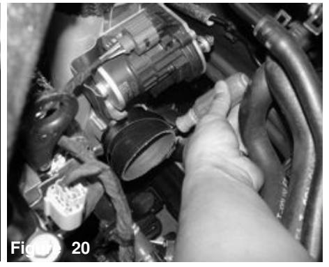
Figure 17 Re-install the inlet duct and make sure the slot of inlet duct lines up with the slot on the air divert. Arrow indicates air diverter and slot indicated in figure 16
