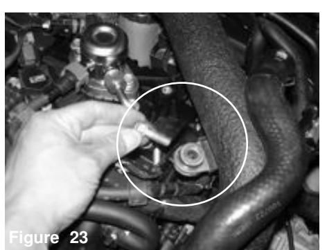
Figure 20 Use a 8mm nut driver and only tighten the #40 clamp on the 2.50" side of the step hose attaching the step hose to the turbo inlet
