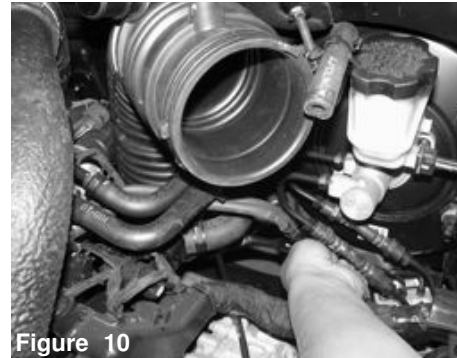
Figure 7 Loosen the clamp on the intake air duct connected to the air box assembly. Detach the intake air duct from the air box assembly
