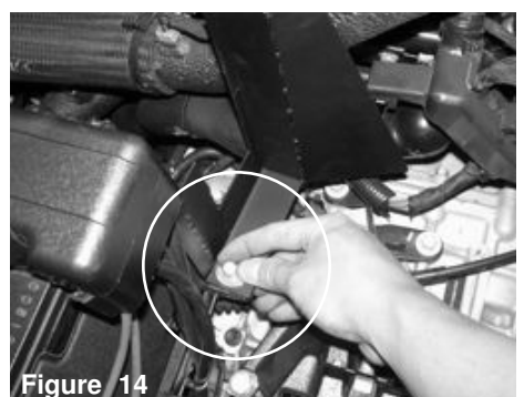
Figure 11 Detach the intake air duct from the turbocharger and you may now remove the intake air duct from the engine bay.
