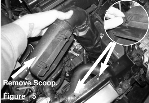
Figure 5 Remove the 2 push clips from the front of the radiator support holding in the ram scoop and then remove the air scoop.
