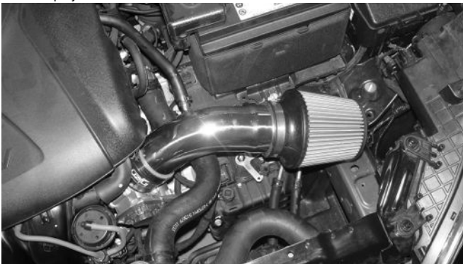
This intake system can be converted short ram for emergency situations.
