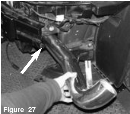
Figure 27 The intake pipe will be inserted from the bottom, behind the bumper support.
