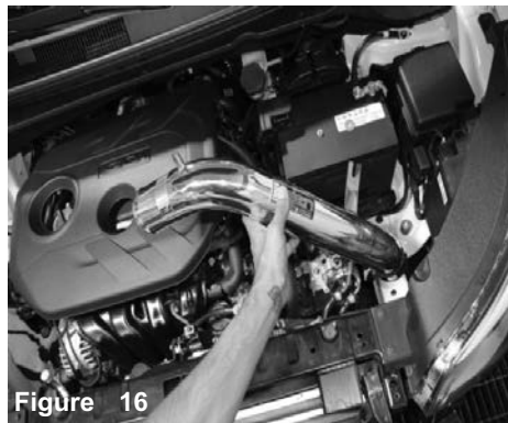
Figure 16 Install the intake into vehicle and position tube to hose and bracket to the vibramount
