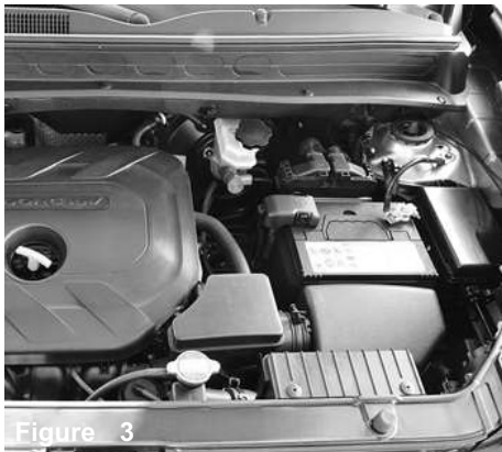
Figure 3 Stock OEM intake system.
