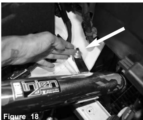
Figure 18 Position for the best fit. Secure the bracket using provided m6 nut and fender washer.
