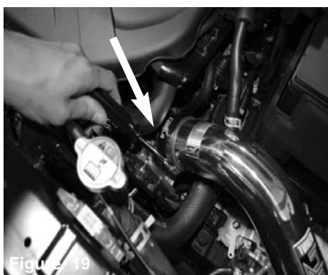
Figure 19 Tighten all clamps using 8mm nut driver.
