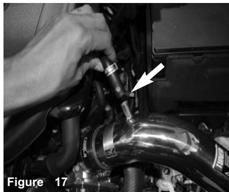
Figure 17 Position the crank case line to the fitting on the intake tube. Secure using the factory clamp.
