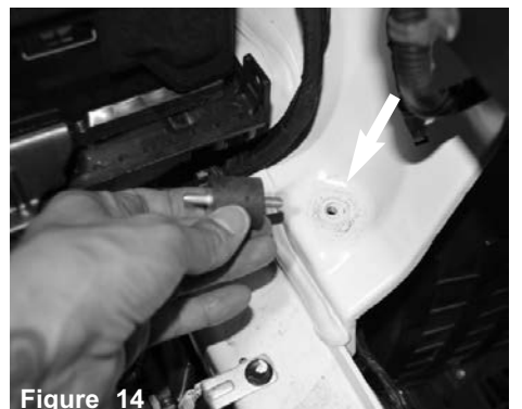
Figure 14 Install the vibramount to the threaded insert on frame.
