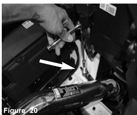
Figure 20 You may now tighten the M6 nut to secure the intake bracket to the vibra mount.
