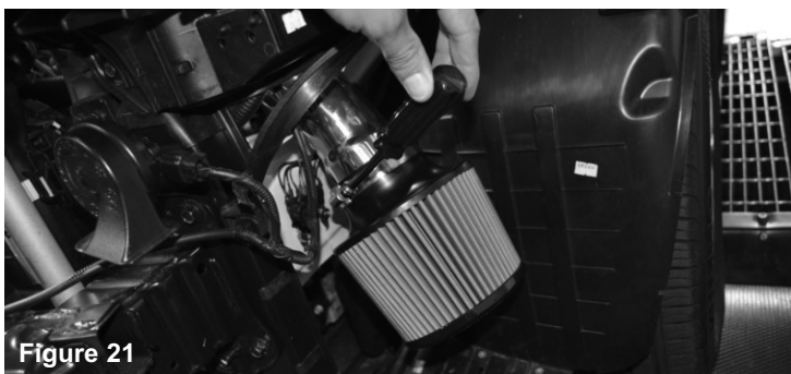
Figure 21 Place the filter onto the end of the intake pipe. Tighten the clamp on the filter with a 8mm nut driver to secure the filter to the intake pipe.
