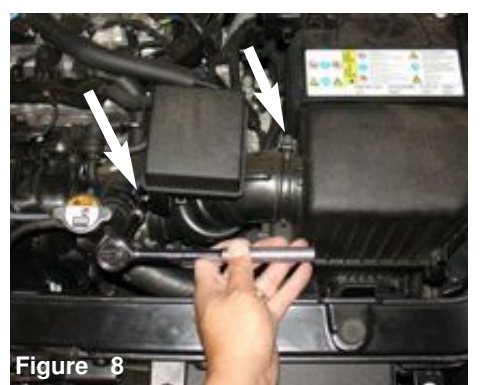
Figure 5 Use a 3/8 -10mm socket with extension and ratchet and loosen the two 10mm bolt on the air box assembly.
