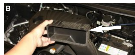
Figure A: Use a phillips screw driver and remove the two plastic retaining screws on the front vent duct. Figure B: This air duct will be removed.
