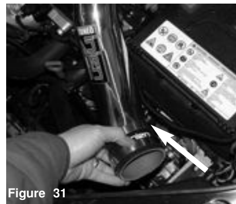
Figure 28 Once you have connected the crankcase vacuum line, continue to slide the tension clamp over the end of hose..
