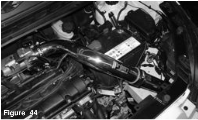
Figure 41 The filter is now inserted into the driver side corner bumper, the filter neck is aligned to the intake.
