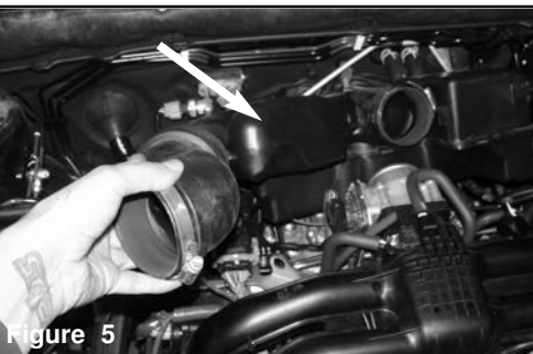
Figure 5 You may now remove the entire air duct assembly
