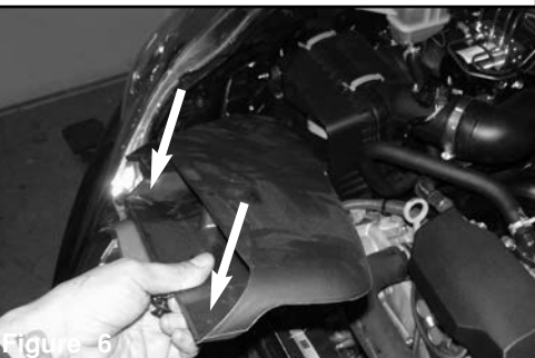
Figure 6 Remove the two plastic retaining clips indicated by the arrows and then remove the front air scoop.
