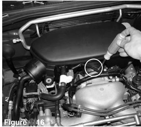
Figure 16 With 8mm nut driver, loosen the clamp holding in plenum box on throttle body.
