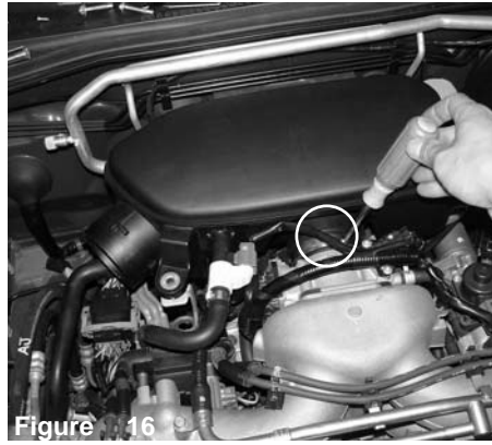
Figure 16 With 8mm nut driver, loosen the clamp holding in plenum box on throttle body.
