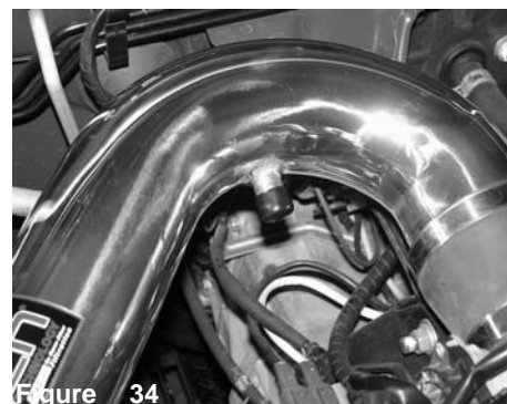
Figure 34 2005 model only cap off the 5/8 fitting.
