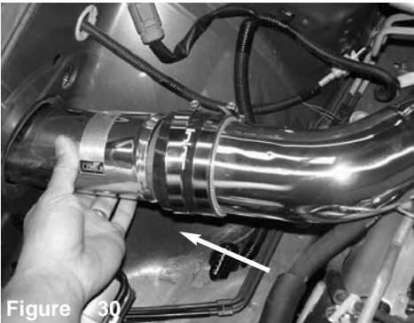
Figure 30 Secure lower intake tube to vibra mount using provided M6 fender washer and nut.
