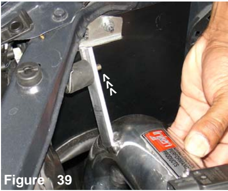
Figure 39 The intake bracket is aligned to the vibra-mount stud.
