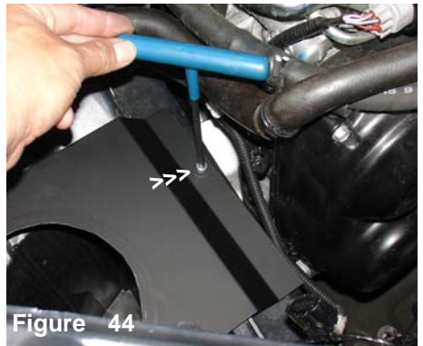
Figure 44 An allen wrench is used to tighten the bolt on the heat shield.
