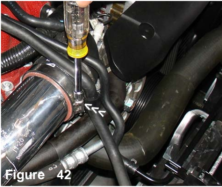
Figure 42 Once the intake has been properly aligned, continue to semi-tighten the power clamp.
