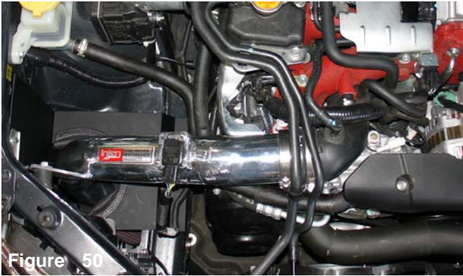
Figure 50 Congratulations! You have just completed the installation of the best cold air intake on the market. Periodically, check the fitment of the intake, normal wear and tear on the engine may cause shifting of the intake system that may cause damage to the intake.
