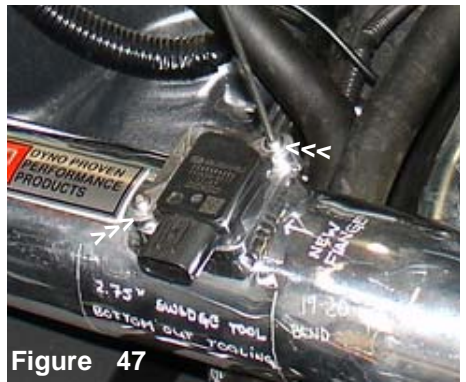
Figure 47 An allen wrench is used to tighten the stock screws on the mass air flow sensor.
