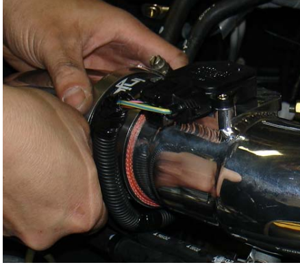
Insert intake end into the inlet side as shown above. Adjust the intake bracket to the vibra-mounts stud and semi-tighten clamp.
