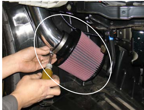
Slip the filter over the end of the intake until it butts up against the stop. Tighten the filter neck clamp to prevent the filter from slipping off.
