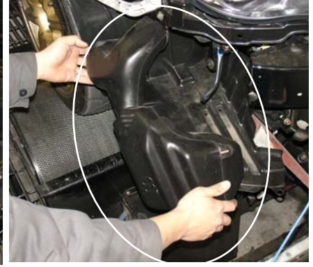
This installation will require the removal of the front bumper. Once the front bumper has been removed continue to pull out plastic resonator box as shown above.
