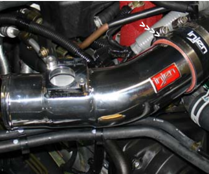
Take the primary intake and press the 3" end into the inlet hose as shown above. The clamp is semi-tightened to hold the intake in place.
