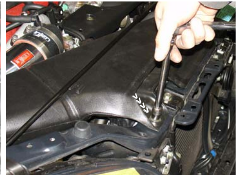
Once you have completed the installation and aligned the intake for the best possible fit, continue to tighten all nuts, bolts and clamps. Place the air scoop back to its original position and tighten the bolts.
