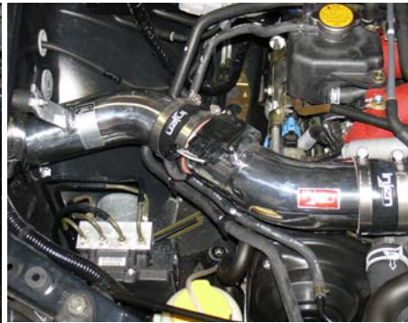
The entire cold air intake is now installed. Continue to adjust the entire intake assembly for best possible fit, prior to moving on to the final instruction.
