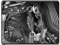
**6.** Locate the 2 threaded studs in the engine compartment, this will be used for the heat shield.
